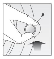
Plastic plugs, supplied inside the protective bag and designated as "P", should be placed in the safety bolt holes according to the direction shown.
